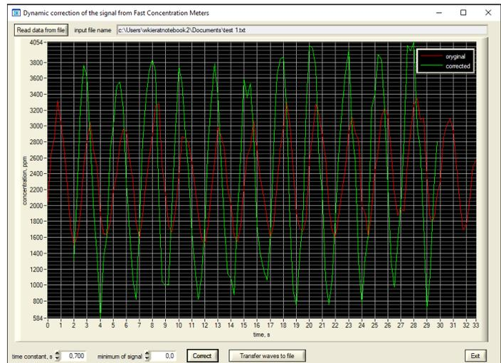
Figure 6 Screen of software used for dynamic correction of recorded measurements.
