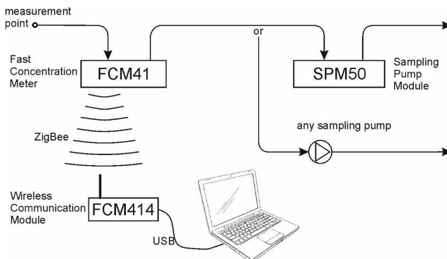
Figure 3 Measuring system connections.
