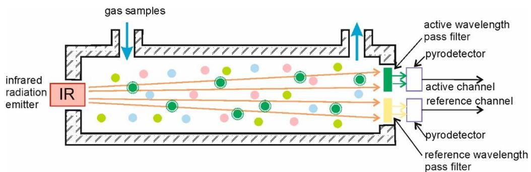
Figure 2 Measurement chamber
