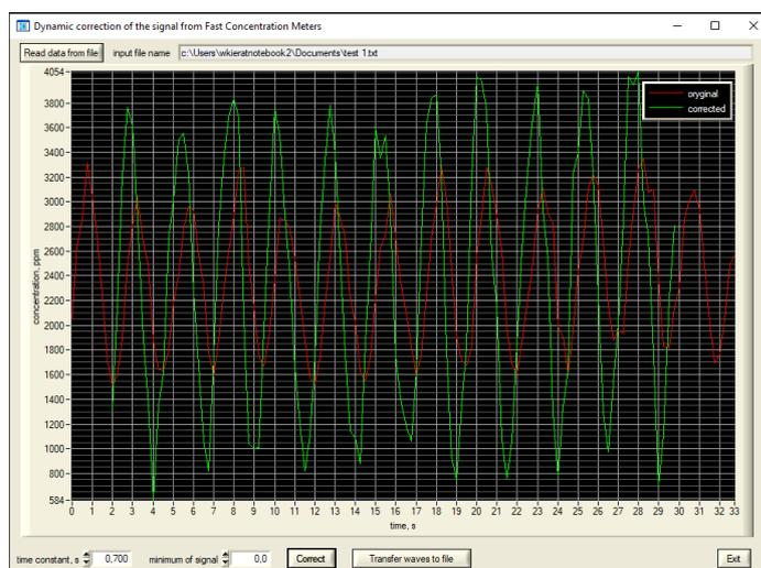
Figure 3 Screen of software used for dynamic correction of recorded measurements.
